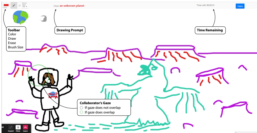
Fig. 1. EyeDraw supports two users, here P21, drawing on a shared synchronous canvas. A gray circle shows the collaborator’s gaze, but here, since both users are looking at the astronaut, it turned green. A simple toolbar with color and brush size controls is available along with the prompt and a countdown timer for the experiment.
