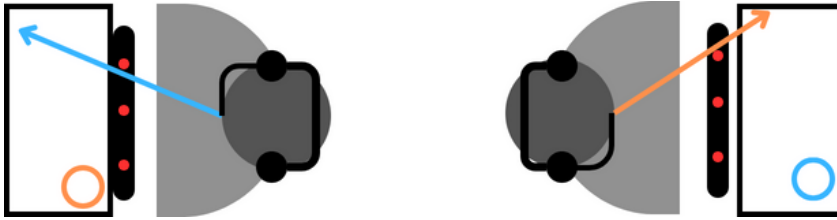
Fig. 2. The experiment set up. Participants wore noise-canceling headsets to communicate during the voice-enabled conditions, V and B, and faced away from each other for the duration of the experiment. Eye trackers were mounted at the bottom of the monitors. The point of gaze of each participant is visualized on their collaborator's screen in real time.
