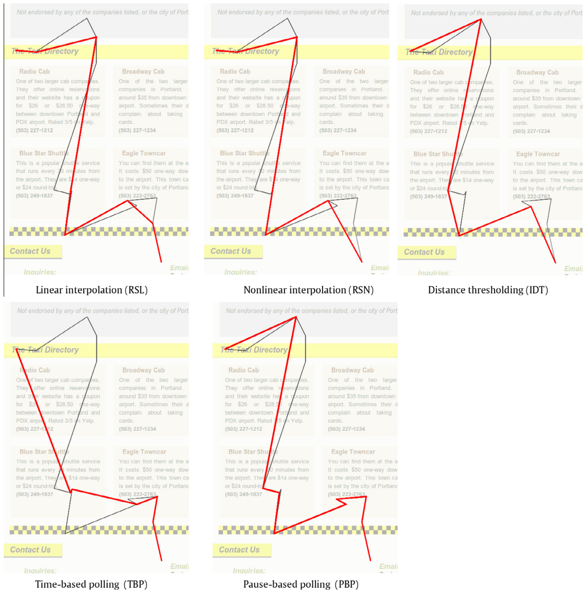
Fig. 3. An illustration of a cursor trail compressed with different lossy compression algorithms in a thick red line, drawn alongside the original cursor trail in gray. The compression ratio for each algorithm is set to 50%, removing half of the original cursor coordinates. (For interpretation of the references to color in this figure legend, the reader is referred to the web version of this article.)
