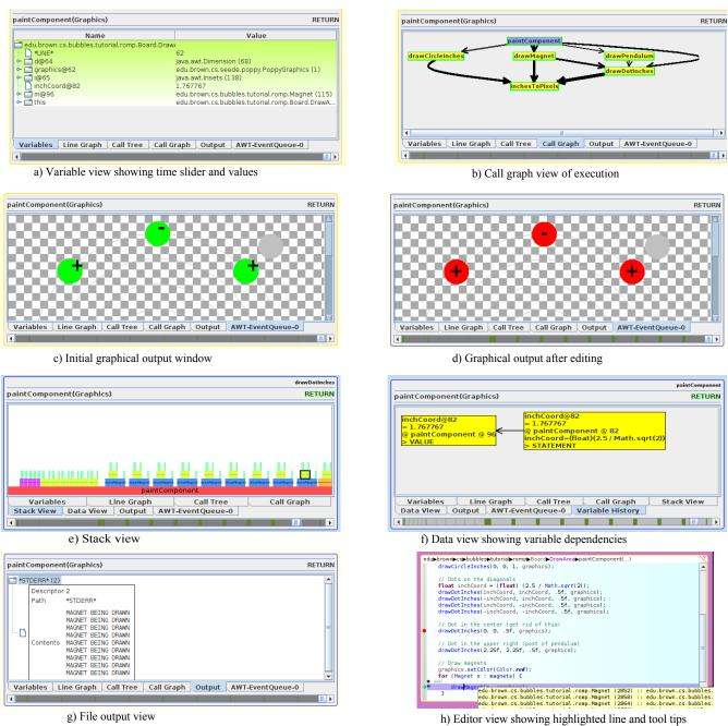
Figure 1: Views of the continuous execution display bubble. The main view (a) shows the variables in the current context. The methods used in the current context are shown in a call graph (or tree) view (b) or in a stack view (d). Graphics output for underlying or user selected component can be displayed (c and d). Variable dependencies for a user selection is available (f), as is the output to files or the console (g). The interface also coordinates with the Code Bubbles editor (h).
